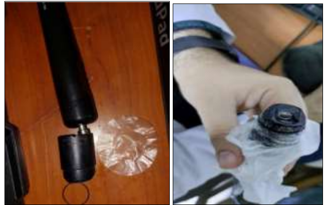
Fig 8: Cap kit offered by Sonoma Escalon company which was consisted of piece of tube covered by plastic membrane surrounded by rubber band
