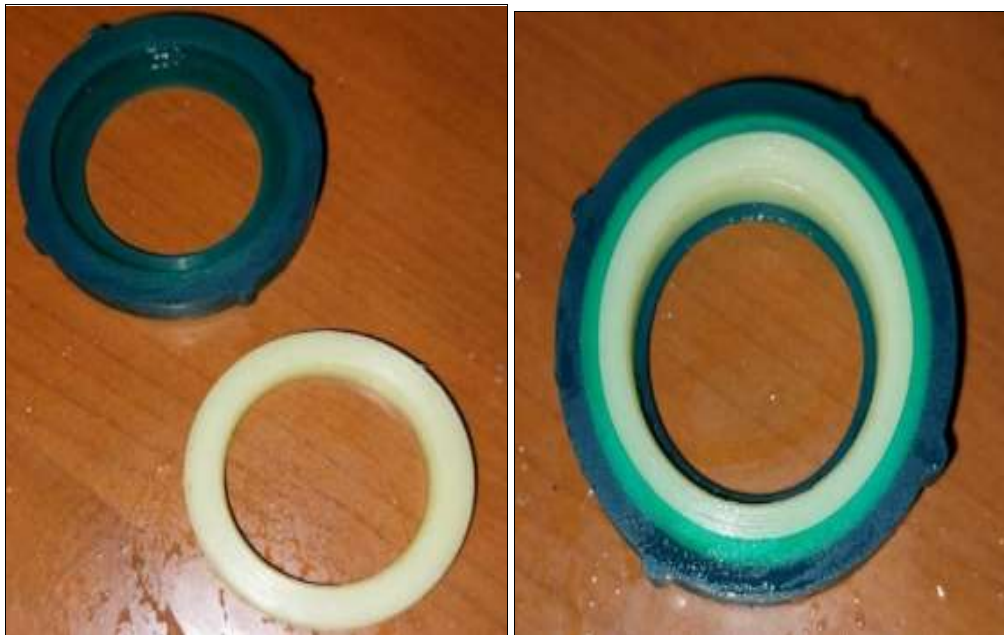
Fig 5: A ring from Teflon material was covered by rubber ring to fix it
