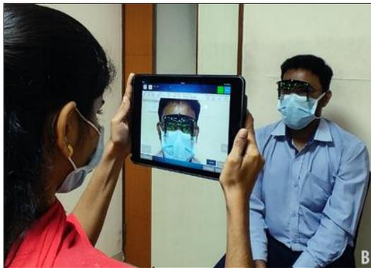
**Fig 1B:** IPD measurement using the commercially Non-Contact Digital IPD measuring Device
